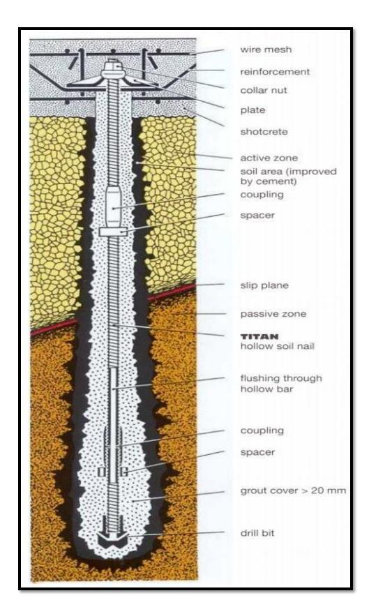
Figure 4: Soil nailing details
