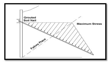
Figure 3: Stress distribution of soil nail
